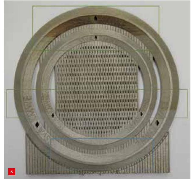
1. There was some deformation on the bottom of both seals (see the area marked in blue in Figure 6, and Figure 7). A cause could not be determined immediately, although shrinkage of the material was suspected. After analysing the print job, the new slicer and its new parameters were found to be the cause. Slicer software is normally used to partition the product in thin layers that are printed sequentially.
