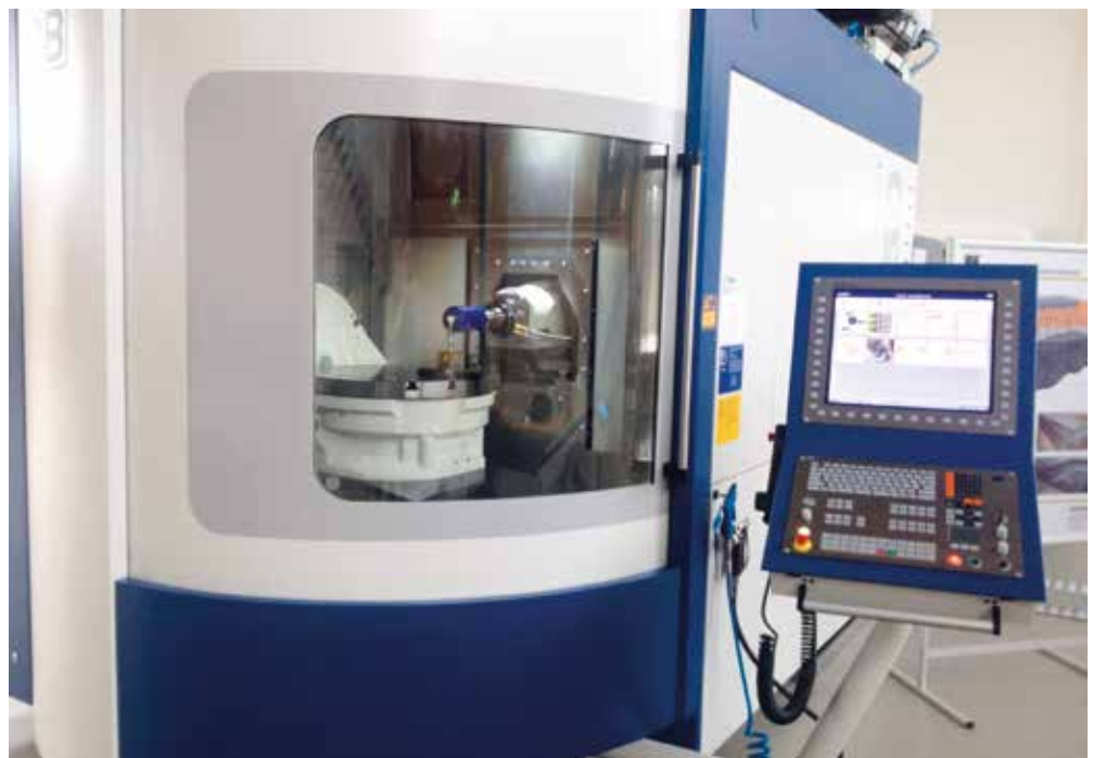
Integration of the Rotary Inspector into a machining centre.
